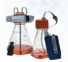
The sensor system can display the relevant growth behavior and metabolic state of the cell culture over a certain time range (21 days). Data is generated at a frequency of 20 seconds/time, and your cell culture status is observed throughout the day. It is also possible to connect directly to the OPC server for process feedback control through on-line monitoring of glucose consumption and lactic acid production.
